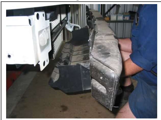
Shown removing bumper cover support with plastic under guard
