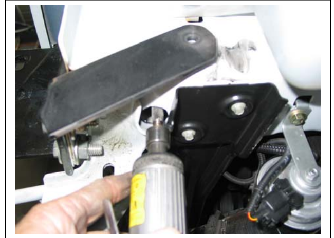
Shown die-grinding passenger side lower hole.
